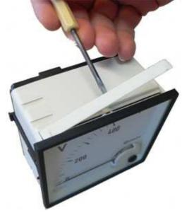
4. Now enter the srewdrivers` head into the slot at the upper edge of the scale ...
