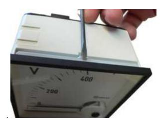
5. ... and pull it out slowly in upward direction. By doing so take care not to contact the pointer of the instrument with the scale.
