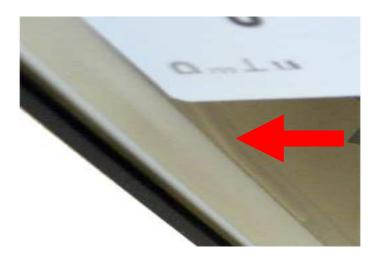
7. Especially at the moment when the scale is passing at the pointer pay attention that pointer and scale do not get in contact to each other. Otherwise the pointer could get deformed.
